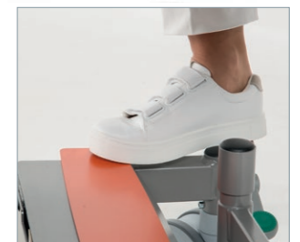
Emergency foot switch
